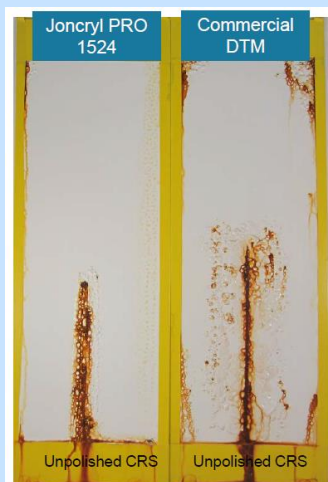
White DTM Salt Spray Test Results after > 322 hours on Cold Rolled Steel. (40-50 µm dry film thickness)
